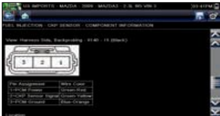
Component locator and connector diagrams show the best test locations.
